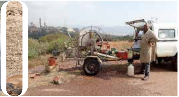
Borehole sampling at the Pelindaba site
