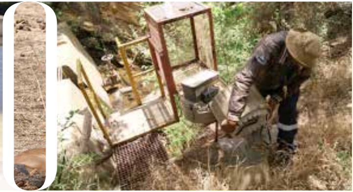
Collecting boundary stream water from an autosampler
